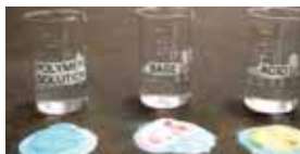
The Indicator function shows kind of spilled substance
